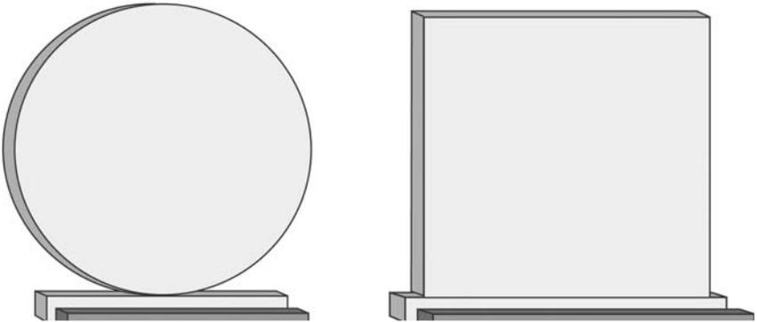
**Measurement tolerance on steel plates +/- 1/4 inch**
